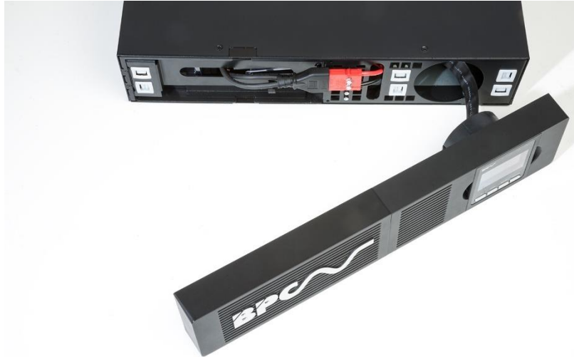
Figure3.8 Removing front facia – Display side first
