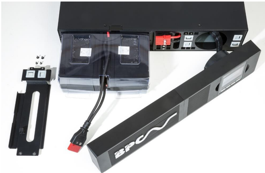
Figure3.9 Battery internal Anderson connector
