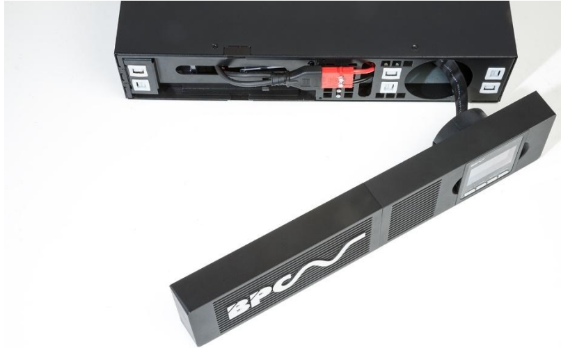
Figure3.8 Removing front fascia – Display side first
